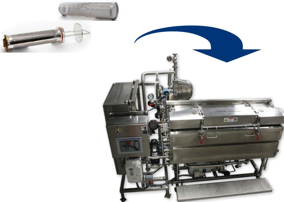
**Figure 3: Example Cleaning in COP Immersion Parts Washer**
