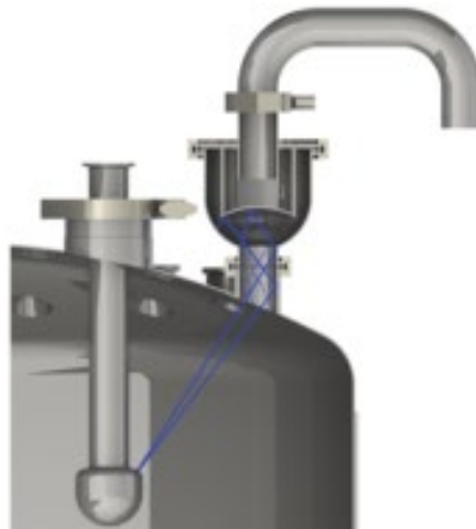
Figure 2: Installation of HSD
