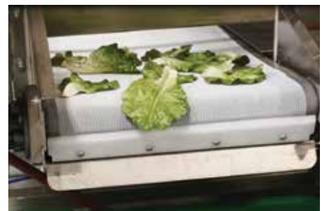
Automated Conveyorized Mesh Screen - Outside View
